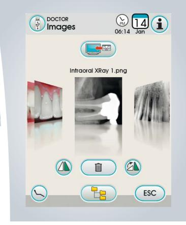
X-rays obtained with a digital sensor can be displayed quickly and simply, directly on the Full Touch control panel. The display provides users with high quality diagnostic images and, thanks to advanced Skema 6 electronics, dentists can correct brightness, adjust contrast and size and set up an X-ray folder in the patient's medical records by saving images on the control panel itself or on an external drive via a USB port.
