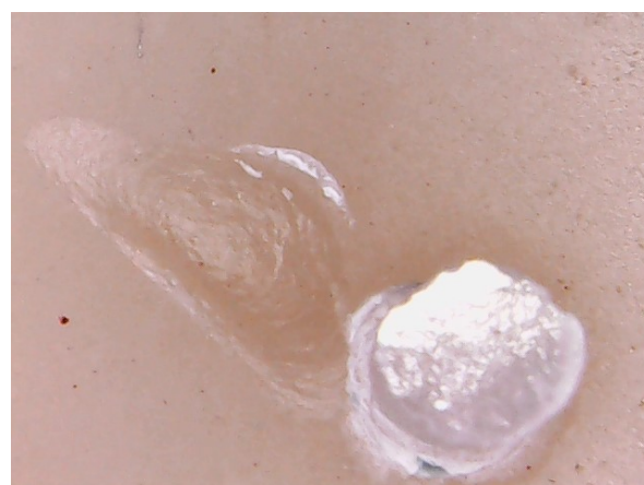
Figure 2. Failure mode distribution after bond strength test after 24 h of storage. The failure mode after 6 months of storage was adhesive type for all groups.
